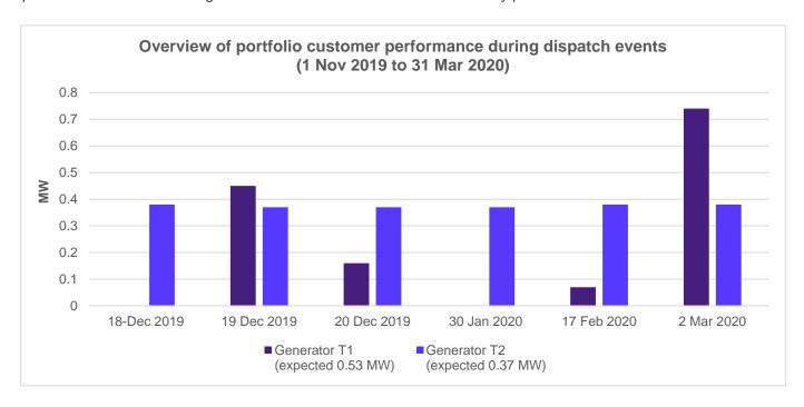
As can be seen from the chart, generator T2 performed very well. It has consistently provided a firm output of approximately 0.38 MW during all dispatch events. However, the other generator, T1, has not always run as expected. The reasons for this are discussed below.
