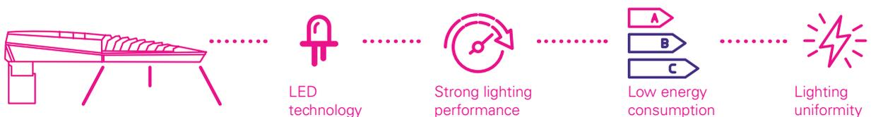
Designed and patented by Enel Sole, the Archilede range of products is marked by strong **lighting performance**, low energy consumption and lighting uniformity. LED technology guarantees energy savings of up to 80%. The devices' service life can reach and even exceed **100,000 hours** without any planned maintenance, thanks to the use of high-quality LED and internal temperature control systems.
