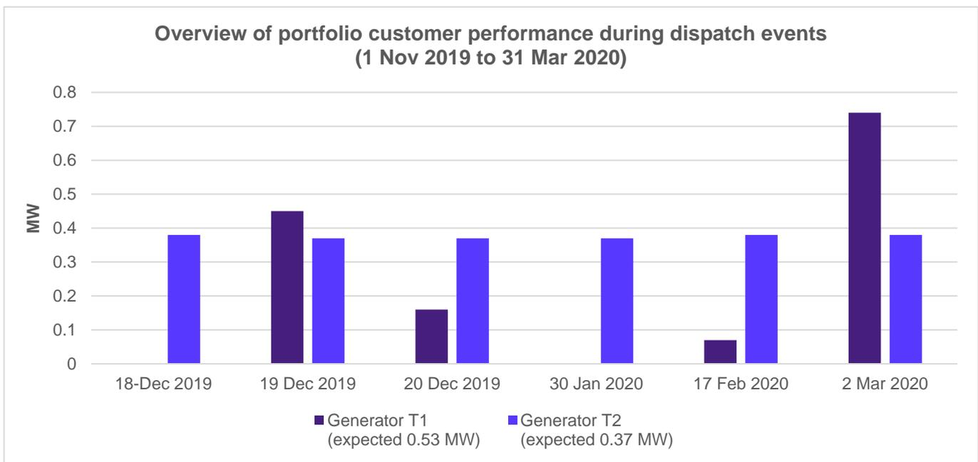
As can be seen from the chart, generator T2 performed very well. It has consistently provided a firm output of approximately 0.38 MW during all dispatch events. However, the other generator, T1, has not always run as expected. The reasons for this are discussed below.
